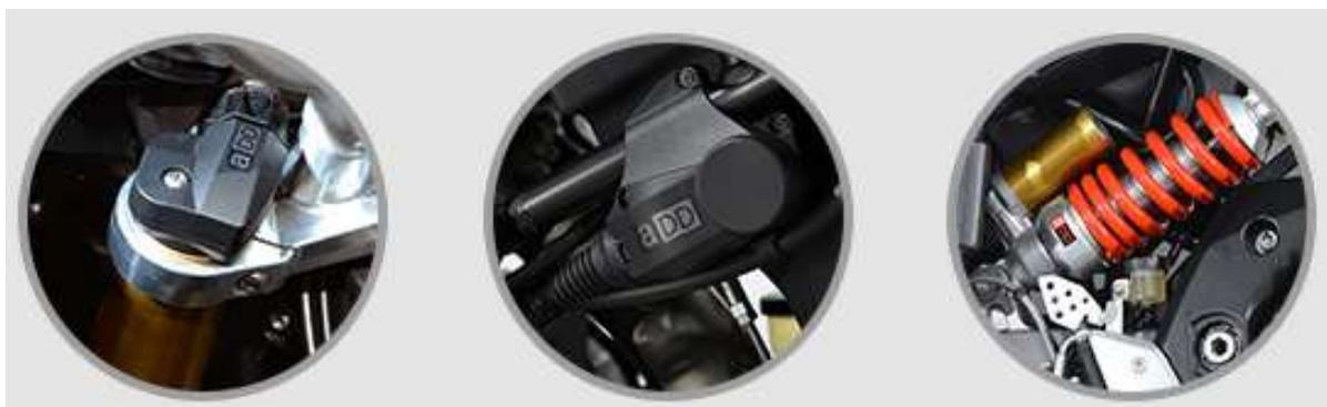
The system recognises different riding phases (**acceleration, throttle release, braking, constant throttle**) and adjusts the baseline fork and shock absorber settings thanks to yet another patent which allows specific hydraulic calibration curves to be defined within the adjustment range.
