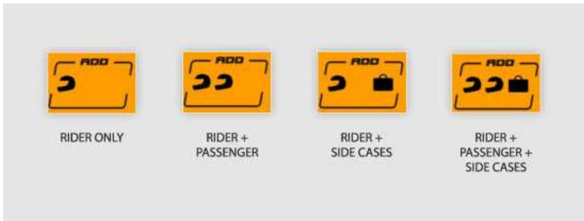
The ADD package also includes a built in piggy back shock absorber which is electrically adjustable in spring preload to **4 predefined settings**, indicated by specific icons on the digital instrument panel: rider only, rider with passenger, rider only with panniers and rider and passenger with panniers.
