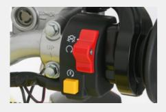
Rider-friendly electric engine starter with compact electric starter motor.
