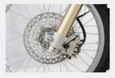
250mm front disc brake with Nissin dual-piston caliper and 220mm rear disc brake with single-piston caliper.
