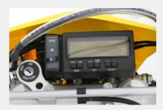
Easy-to-read multi-function digital instrument includes speedometer, odometer, dual tripmeters with both addition and subtraction functions, clock and stopwatch with subtraction capability.
